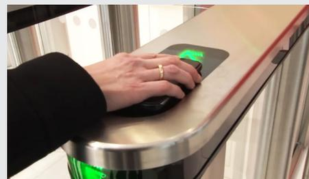
The entry into the building and sensitive areas are managed in real-time and can be done with DESFire badge or a SIM NFC smartphone.
