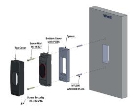
The narrow model (XS), shown above, can be installed with a spacer (ref. SOC05HR1000-N). This spacer, fixed to the wall with 2 screws, is necessary for the operation of the infrared anti-tear device, and facilitates the installation of cables and connectors.
